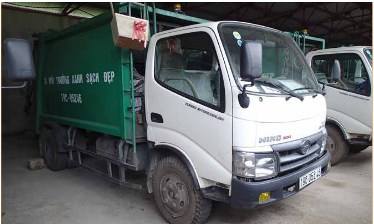
FIGURE 2-16 Typical small compaction truck used for secondary collection and transportation
